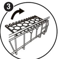
Cup rack folded out ... .. or raised upwards
